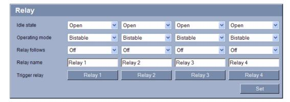
You can configure the switching behavior of the relay outputs. For each relay, you can specify an open switch relay (normally closed contact) or a closed switch relay (normally open contact).
